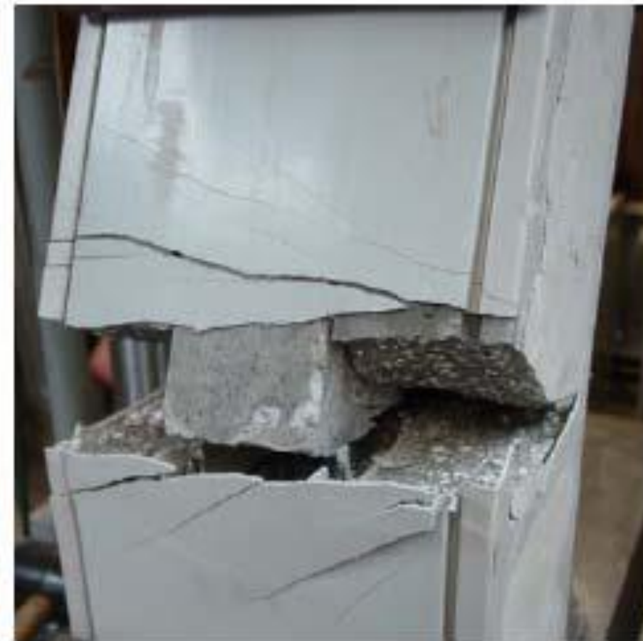
(b) Failure @ 2 in./sec Stroke Rate
